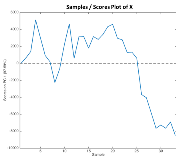
Figure 10. Component 1 of the process example. Horizontal axis is days. A drastic change after 25 days can be noted.
